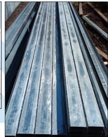
To prevent rejection of material, every precaution should be taken to avoid storage stain on galvanized sheet. Also, specific practices have been developed that allow the shipment and storage of galvanized sheets without the formation of storage stain.
